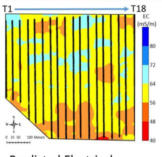
Predicted Electrical Conductivity, Wet, VI + Raw bands, R<sup>2</sup> = 0.49, MAE = 4.2
